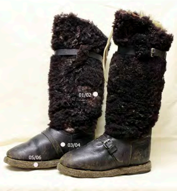
Fig. 10 and 11: Locations of points for XRF measurements. © DHM (BZ_DHM_0107)
