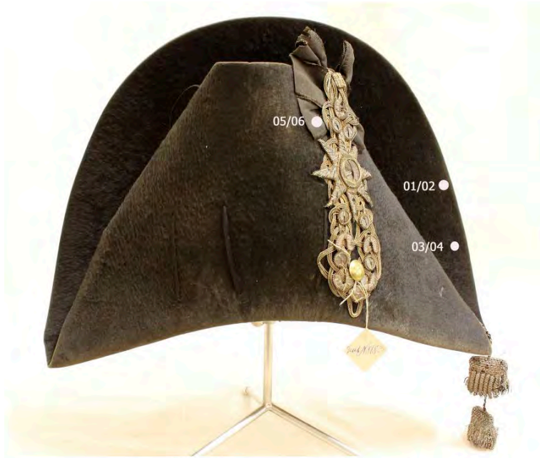
Fig. 4: Locations of points for XRF measurements. © DHM (BZ_DHM_0032)
