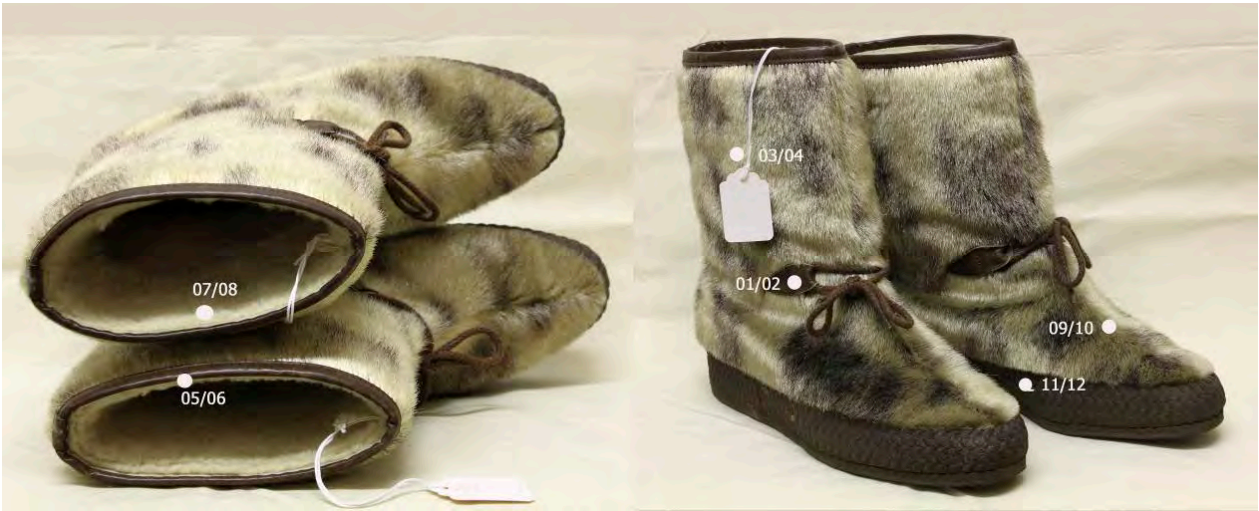
Fig. 12: Locations of measurement points for XRF on inside and outside. © DHM (BZ_DHM_0109)
