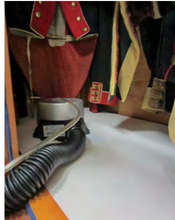
Fig. 8: Air filter measurements, cowling with air filter.
