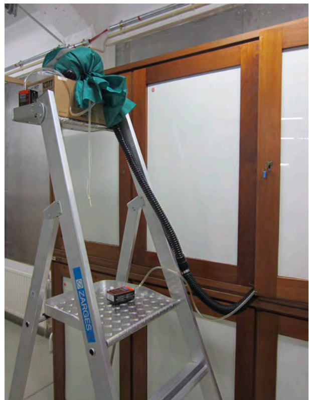
Fig. 9: Measuring filtered air from cabinets beneath duct cawling.
