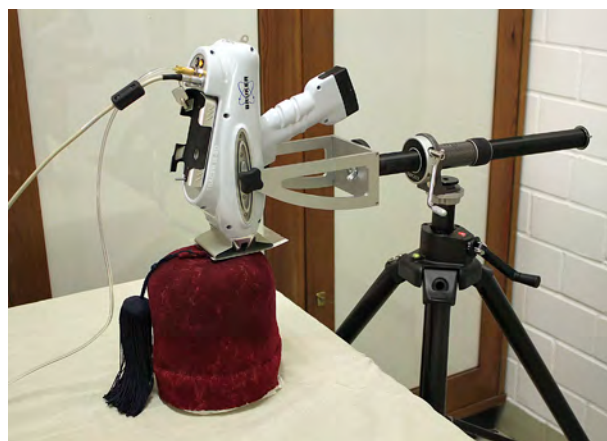
Fig. 1: Examination of a hat by means of X-ray fluorescence analysis.
