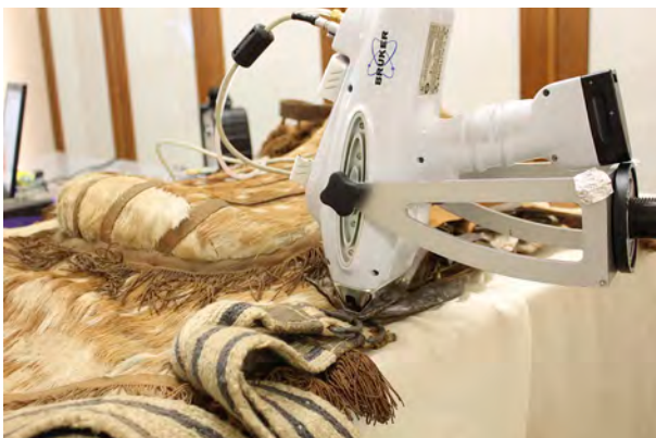
Fig. 10: Measuring with an XRF spectrometer.
