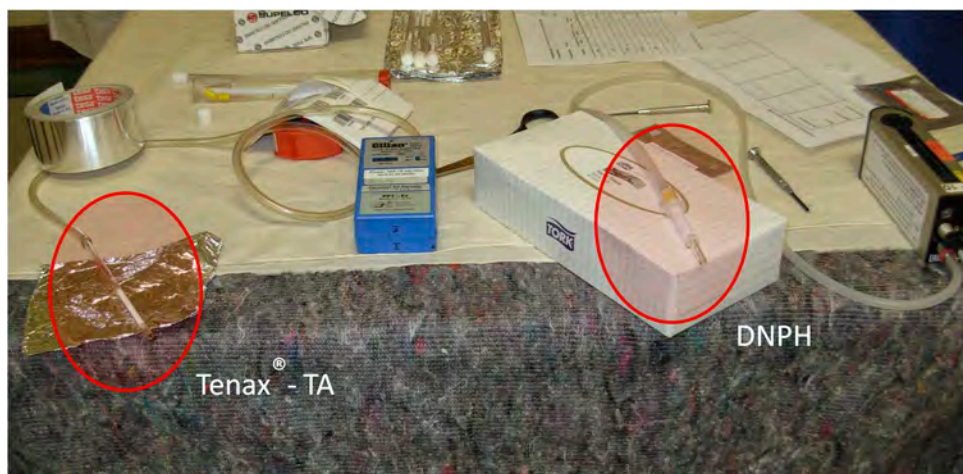
Fig. 2: Room air measurement in the depot of the DHM.
