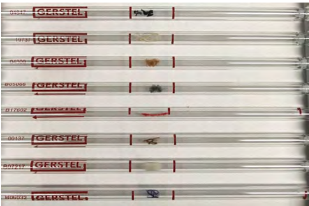
Fig. 3: Glass tube with fiber samples for thermal extraction.
