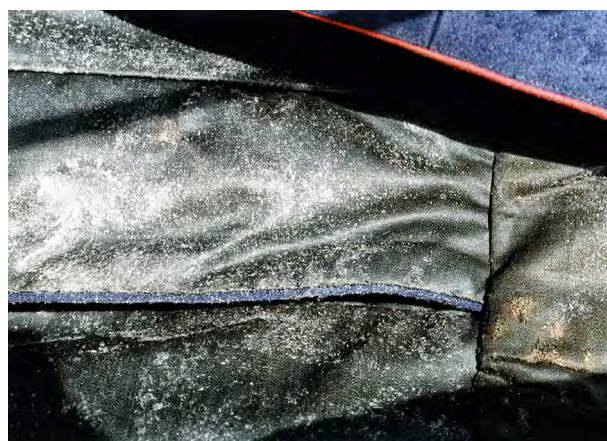
Fig. 3: Crystallized biocide, detail from Fig. 2.
