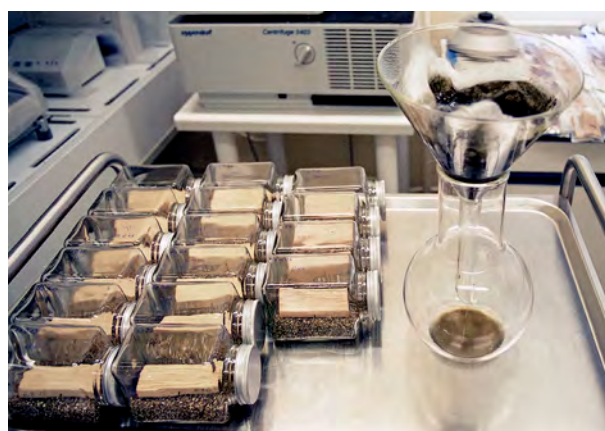
Fig. 2: Left: wood specimens ready to be inoculated with fungal spores of blue stain fungi and to be incubated on water holding granules in the experimental vessel; right: obtaining a fungal spore suspension by filtration of an aqueous extract of sporulating fungal cultures.
